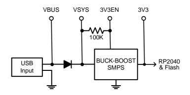
For embedded controller applications generally an external power source (other than USB) is required and this can be connected to VSYS via a Schottky diode. This will allow the PicoMite to be powered by whichever supply is producing the highest voltage (USB or VSYS). The diodes will prevent feedback into the lower voltage supply.
