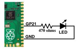
When you have saved and run this program you should be greeted by the LED flashing on and off. It is not a great program but it does illustrate how the PicoMite can interface to the physical world via your programming.
