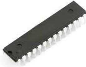
The Micromite is a low cost Microchip PIC32 microcontroller programmed with the MMBasic firmware.
