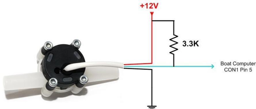
If you use a paddle wheel flow sensor you must check the specifications and only use one that specifically states that it is suitable for use with petrol or diesel fuel. RS Components have a suitable sensor (part nbr 508-2704) and [www.lightflying.com.au](http://www.lightflying.com.au) or [oregonlightsport.com](http://oregonlightsport.com) have a similar sensor made by MGL Avionics.
