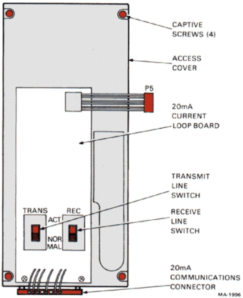
Figure 4-4 Terminal Controller Board
