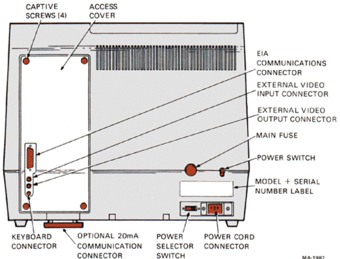
Figure 4-2 Advanced Video Option Installation
