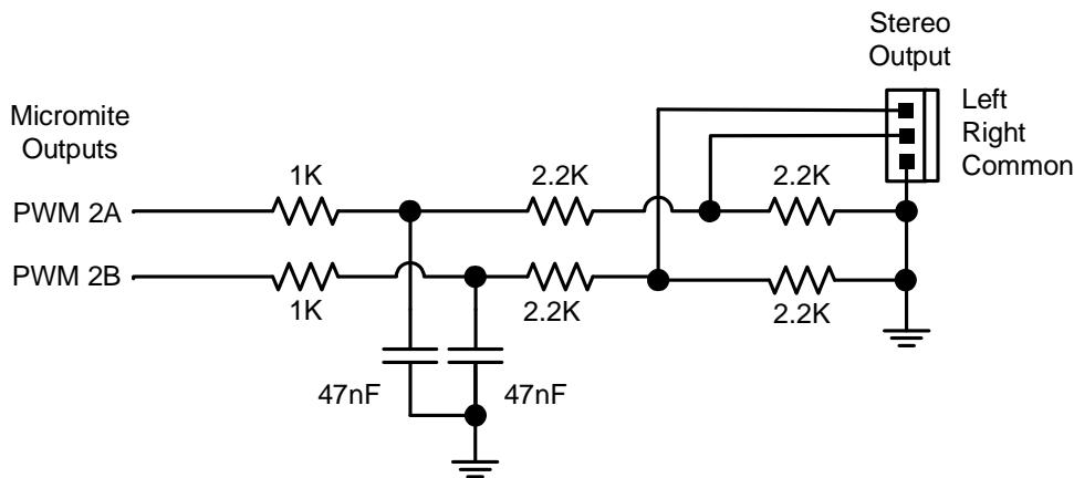
This is suitable for general use, however more sophisticated designs can be implemented if required to improve the frequency response and reject more of the carrier frequency. This circuit is also suitable for generating a DC output signal using the PWM commands although in that case both the 47 nF capacitors should be increased to 4.7  $\mu$ F.
