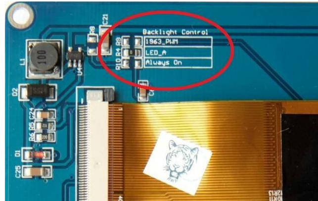
However, it is better to use the SSD1963 controller to generate this signal as it frees up one I/O pin and it allows the brightness to be controlled with a finer degree of resolution (1% instead of 5% steps). To use the SSD1963 for brightness control the zero ohm resistor should be removed from the pair marked "LED-A" and used to short the nearby pair of solder pads marked "1963-PWM". The Micromite Plus can then control the brightness via the SSD1963 controller.
