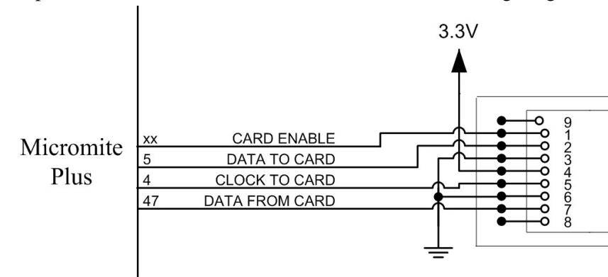
Care must be taken with display panels that share the SPI port between a number of devices (SD card, touch, etc). In this case all the Chip Select signals must be configured in MMBasic or alternatively disabled by a permanent connection to 3.3V. If this is not done any floating Chip Select signal lines will cause the wrong controller to respond to commands on the SPI bus.
